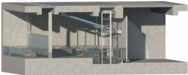
Intelligent Diversion Well / Tilting Gate Type
